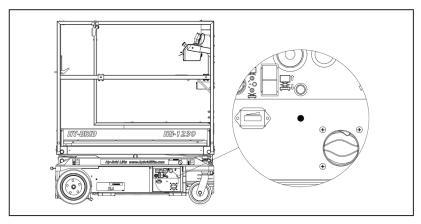
FIGURE 21: Battery Charger LED Display
