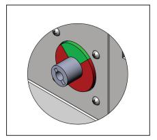
FIGURE 18: Main Power Switch Knob Removed
