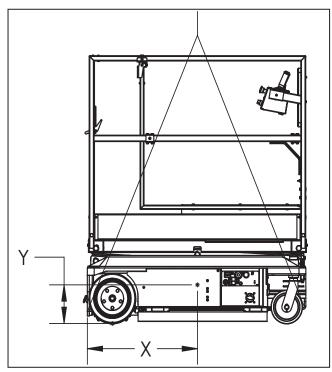
FIGURE 13: Center of Gravity
