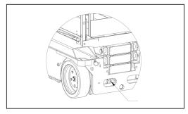
FIGURE 9: Brake Release Handle Location
