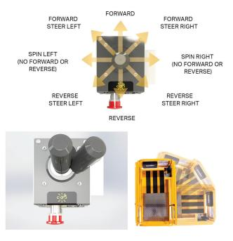
Understanding the difference between Spin and Turn on the Hy-Brid HB-830/HB-1230 is essential for proper machine control and avoiding unwanted caster movement.
