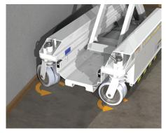
Instead, use spin to rotate the casters away from the wall before traveling
